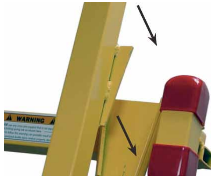
11. PLACE THE TAPERED PLATES OF THE CROSS ARMS INTO THE TAPERED SOCKETS ON THE CRADLE. THE SPRING TAB ON THE BACK OF THE CROSS ARM WILL LOCK IT INTO PLACE.
