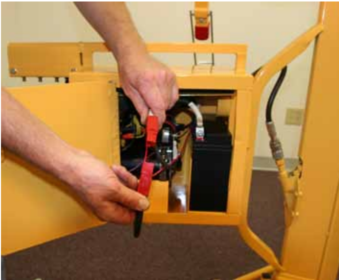
8. OPEN POWER BOX AND CONNECT BATTERY USING EASY CONNECT WIRING HARNESS.
